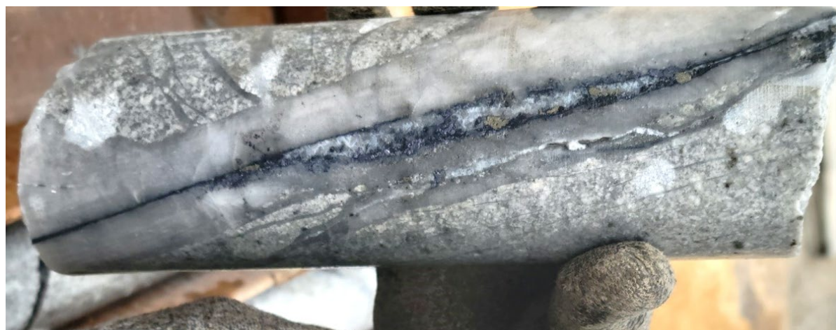
Figure 4: Photo of molybdenite + quartz + pyrite veining within quartz monzonite porphyry stock in drill hole WD22-04 (interval 640.66-642.18m downhole @ 0.22% Mo). 6
