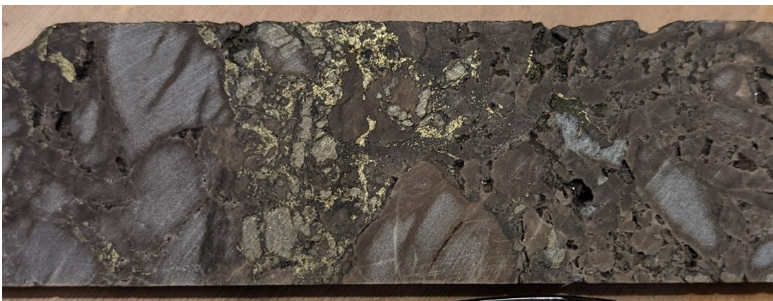
Figure 1: Chalcopyrite (copper sulphide) within Storm exploration drill hole ST22-10 from 313m downhole.
