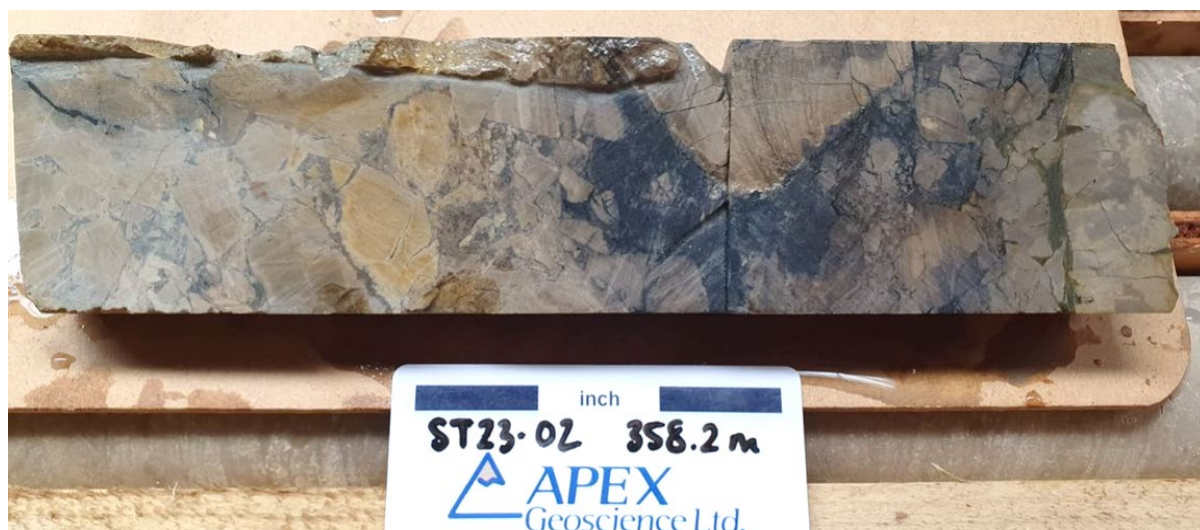
Figure 2: Strong copper sulphide (chalcocite - dark grey) breccia fill and veining in exploration diamond drill hole ST23-02 from approximately 358.2m downhole. This mineralisation is interpreted to be sediment-hosted and is one of five drill holes that have intersected the same prospective unit to date.
