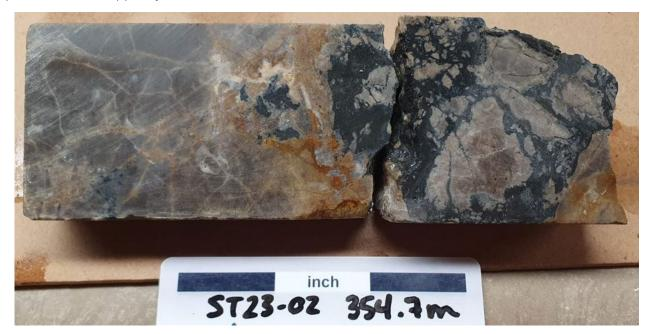
Figure 11: Chalcocite (dark grey) breccia fill in drill hole ST23-02 from approximately 354.7m downhole.
