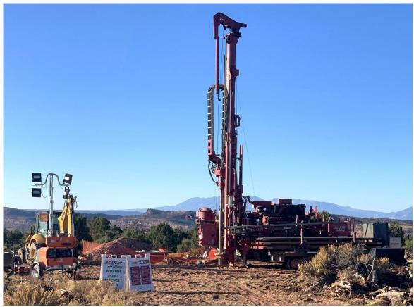
Figure 17: RC drilling at the Copper Warrior Project, Utah.
