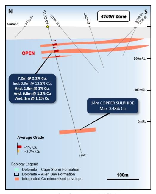
Figure 10: N – S geological section through drill hole ST23-01.
