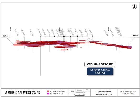
Figure 5: Long section view (looking north at 8174275N) of the Cyclone Deposit and conceptual pit shell.
