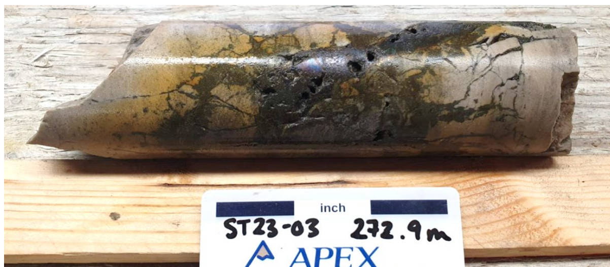
Figure 5: Breccia chalcocite (dark grey), bornite (purple/grey) and chalcopyrite (brassy) in drill hole ST23-03 from approximately 272.9m downhole.
