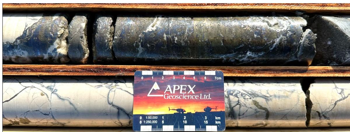
Figure 1: Massive chalcocite (dark grey) and chalcopyrite (brassy) in drill hole ST23-03 from approximately 58m downhole.
