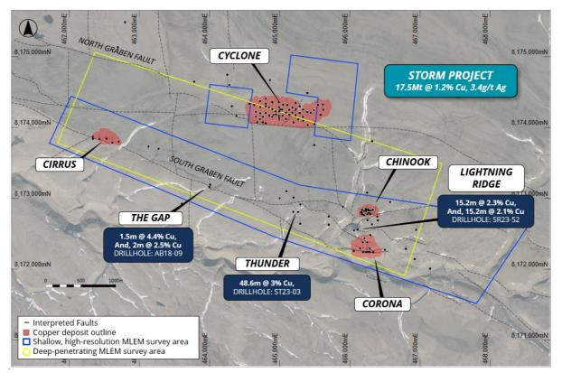
Figure 2: Plan view of the Storm area showing the initial planned MLEM survey areas (configured for shallow and deep exploration) and location of the known copper deposits and prospects, overlaying aerial photography.
