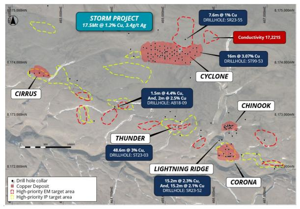
Figure 1: High-priority Electromagnetic (EM) and Induced Polarisation (IP) target areas, current copper resource outlines, overlaying aerial photography.
