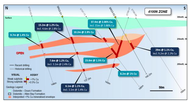
Figure 3: Geological section view at 465,000E showing the interpreted mineralisation envelopes (>0.5% & >1% Cu) and recent drill hole assays and visual observations.
