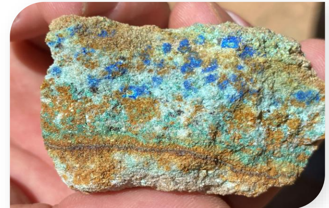
Copper oxides replacing chalcocite in outcropping sandstone.
