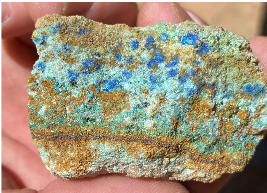
Figure 24: Coarsely disseminated copper oxides (in this case azurite – brilliant blue in colour) are widespread in outcrop throughout the Copper Warrior Project area.
