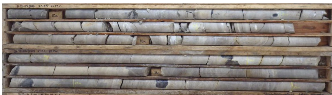
Figure 6: Drill core from ST22-09 between 79.79– 88.15m downhole with dark grey chalcocite veining.
