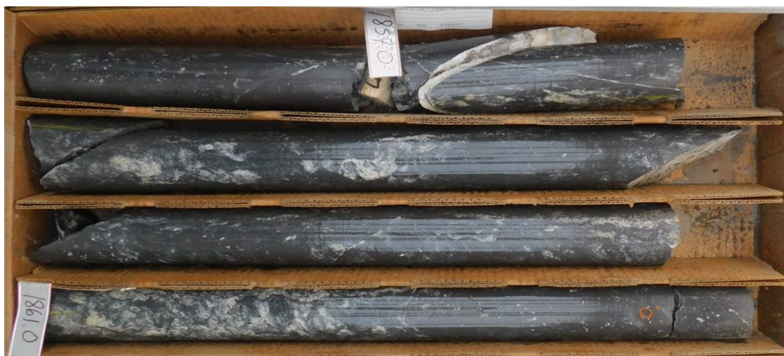
Figure 16: Photo of massive sphalerite (zinc sulphide – black/brown) and magnetite (black) in drill hole WD22-05 at approximately 566 – 567.2m (1857 – 1861ft) downhole.
