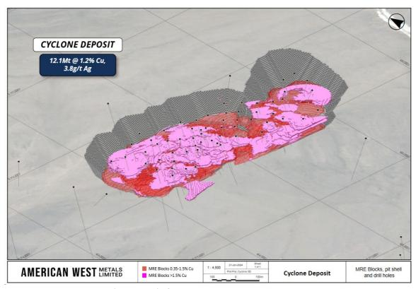
Figure 3: Orthographic view (looking NE) of the Cyclone Deposit and conceptual pit shell.
