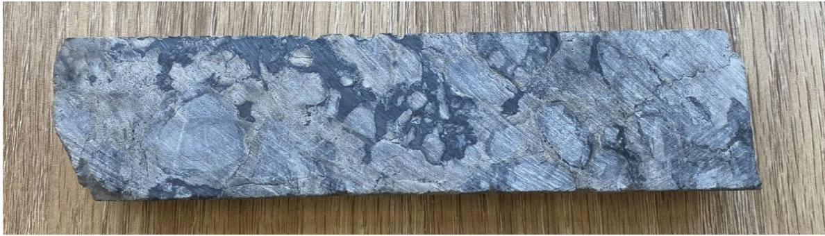
Figure 19: Drill core from STOR1601D from interval 97-101m downhole – average grade 4.16%. The Chalcocite is seen as the dark gunmetal grey material within the lighter grey dolomite host rock.
