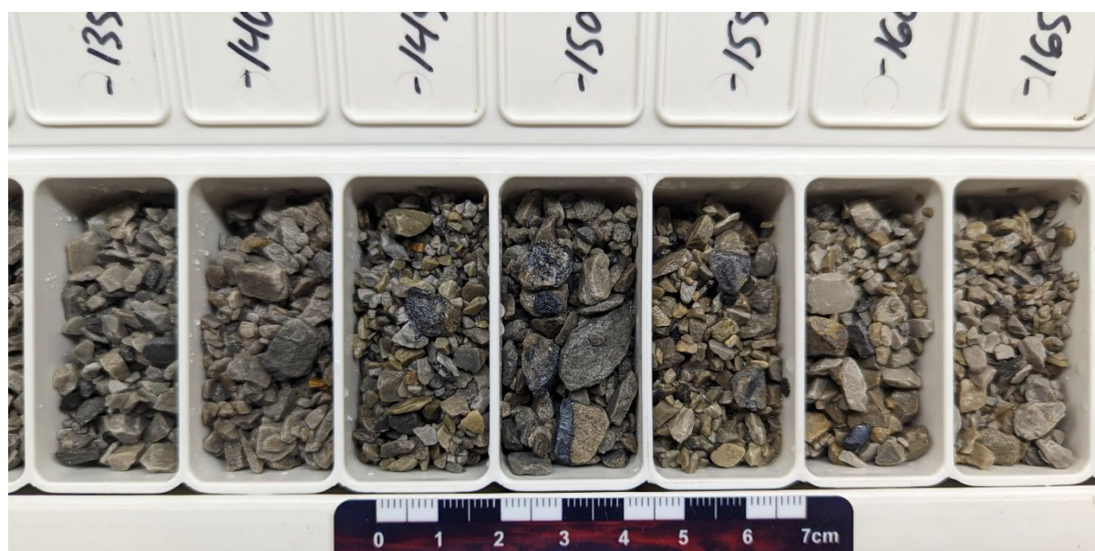
Figure 4: RC drilling chips from SR23-05 between approximately 41 – 50m (135 – 165ft) downhole. Chalcocite (copper sulphide) can be seen as dark gray chips and veinlets.
