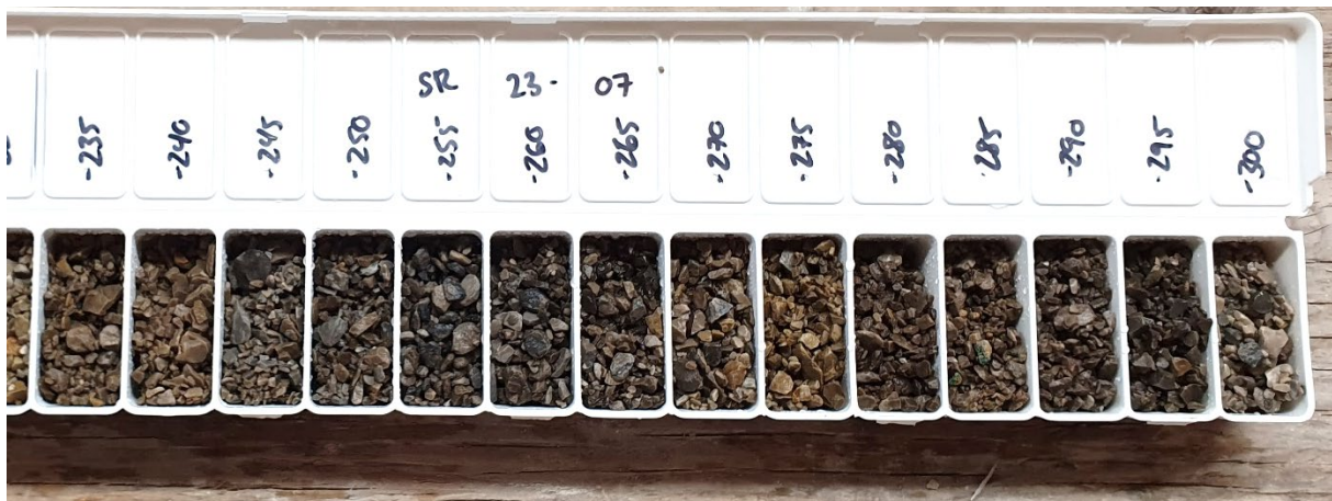
Figure 6: RC drilling chips from SR23-07 between approximately 72 – 91m (235 – 300ft) downhole. Chalcocite (copper sulphide) can be seen as dark gray chips.
