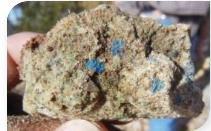
Copper oxides replacing chalcocite in outcropping sandstone.
