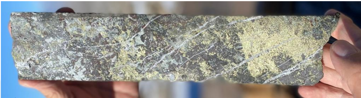
Strong chalcopyrite in drill core from 418m downhole in WD22-01C .
