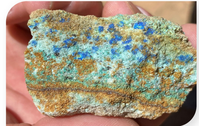
Copper oxides replacing chalcocite in outcropping sandstone.
