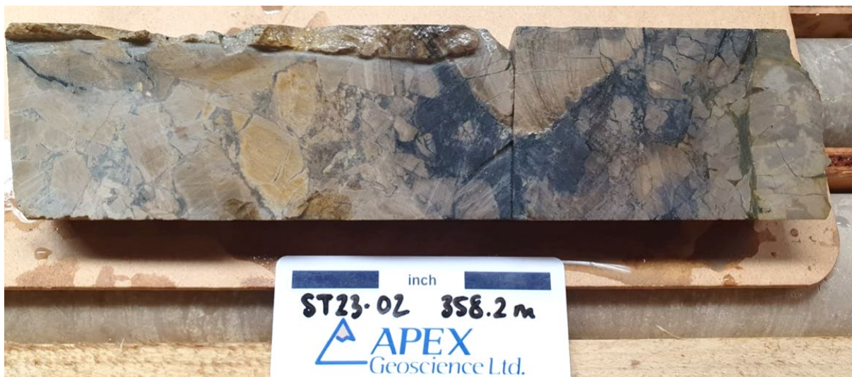
Figure 1: Strong chalcocite (dark grey) breccia fill and veining in drill hole ST23-02 from approximately 358.2m downhole. Chalcocite is a copper sulphide mineral and contains approximately 79.8% copper.
